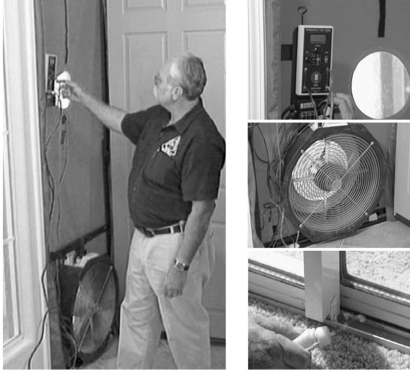
Figure 3-48: Blower Door Testing
